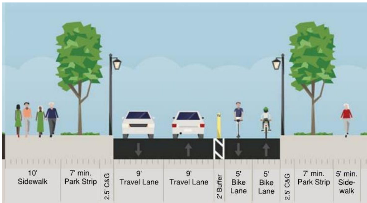
Figure 26: Local roadway (30ft asphalt), separated and plowable 2-way cycle track, and a 10ft multi-use path, reduced on-street parking – 25mph design. Cross section shows only 64ft of 66ft required ROW; widening or adding elements is needed.
