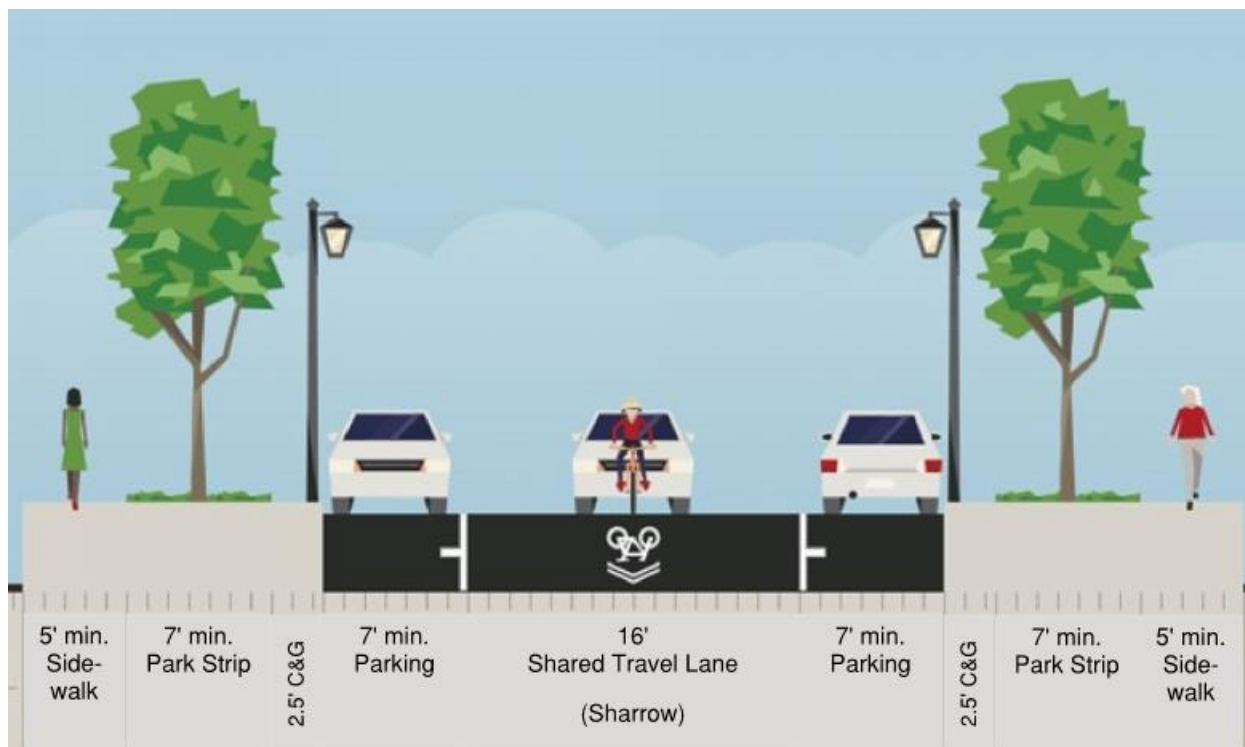
Figure 24: Low volume Local roadway (30ft asphalt- 66ft ROW) – On-street parking with a single “give and go” vehicle and sharrow bicycle lane, creates a true 20mph design. Cross section shows only 59ft of 66ft required ROW; widening or adding elements is needed.
