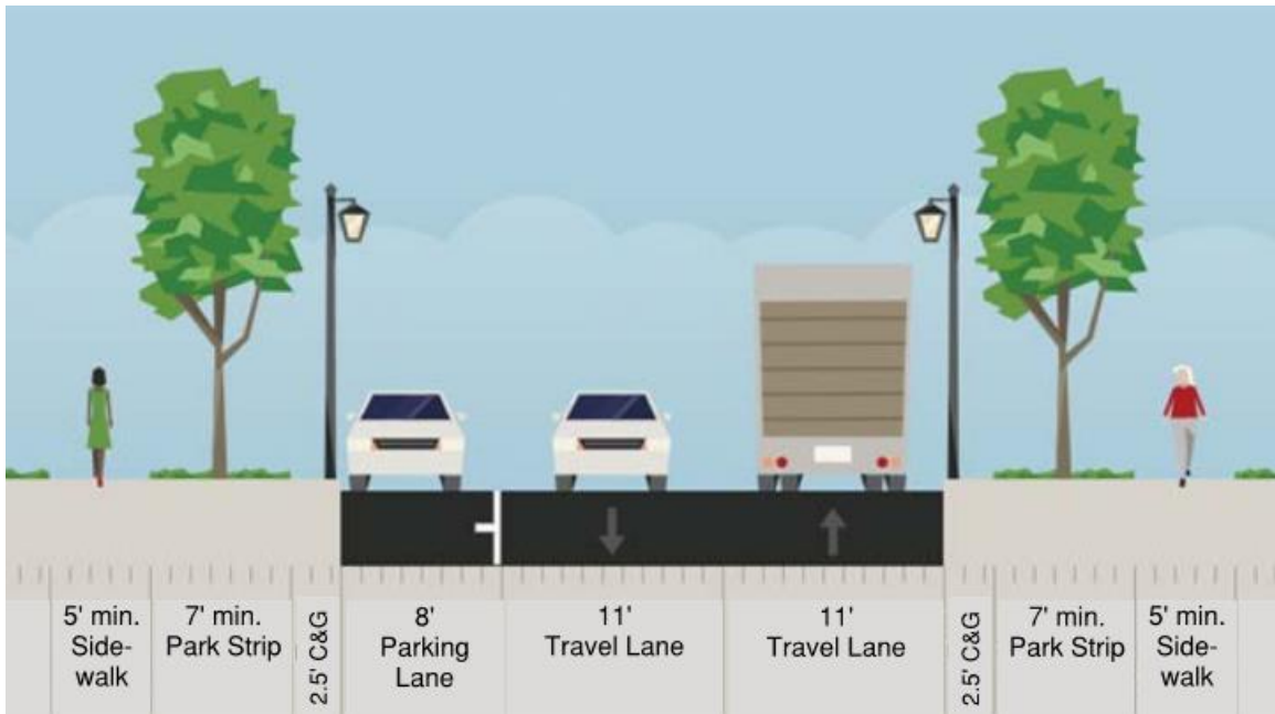
Figure 25: Local roadway/Minor Collector (30ft asphalt – 66ft ROW), two-way continuous traffic and limited on-street parking – 25mph design. Cross section shows only 59ft of 66ft required ROW; widening or adding elements is needed.
