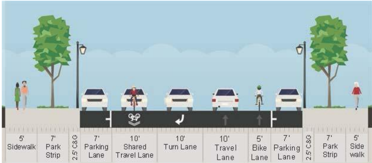
Figure 29: Major Collector (49ft asphalt) with center turn lane, sharrow bike lane and striped bike lane, widen sidewalk as available – 35mph design.
