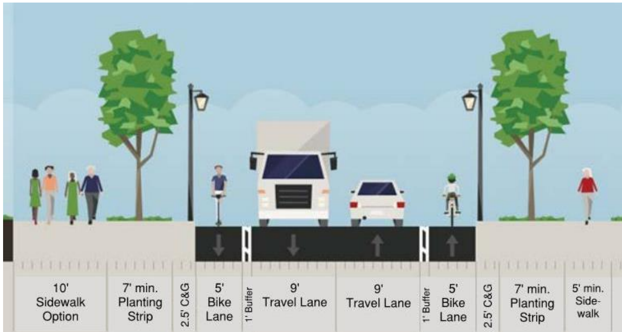
Figure 23: Local roadway (30ft asphalt- 66ft ROW), buffered bike lanes in place of on-street parking and 10ft multi-use path increase active transportation – 25mph design. Cross section shows only 59ft of 66ft required ROW; widening or adding elements is needed.
